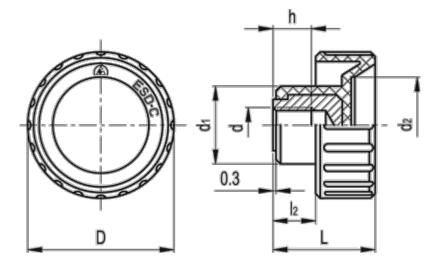
$\begin{array}{lll} D & = 32 \\ d1 & = 17.0 \\ d2 & = 21 \\ d \ 6H & = M8 \\ h & = 10 \\ L & = 22 \\ l2 & = 9 \\ Weight \ (g) = 11 \end{array}$
